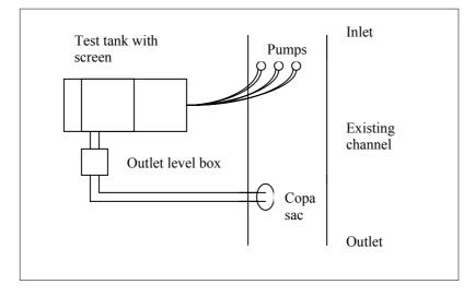
The screens were evaluated one at a time and were placed in a test tank for the measurements. Raw sewage water from the inlet to Floda Wastewater Treatment Plant was pumped up to the test box using one, two or three pumps with a capacity of 12.5 l/s each.
