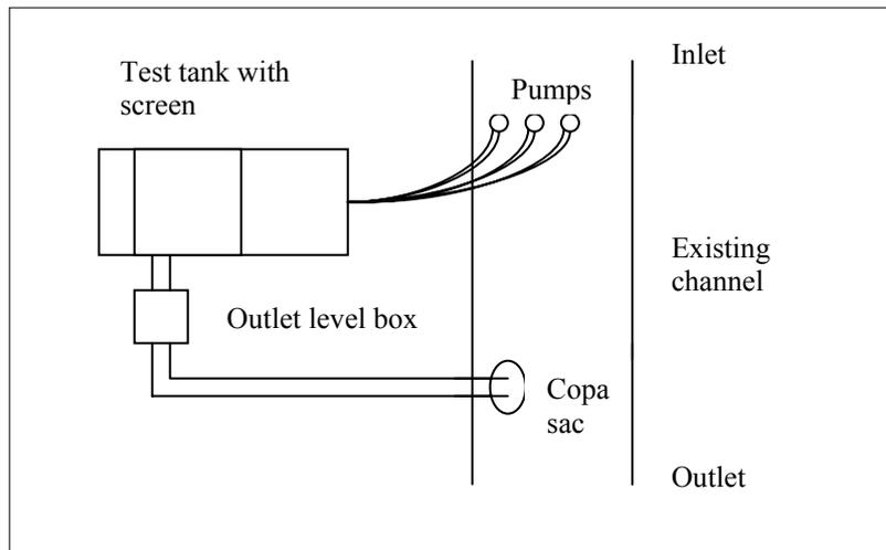
The screens were evaluated one at a time and were placed in a test tank for the measurements. Raw sewage water from the inlet to Floda Wastewater Treatment Plant was pumped up to the test box using one, two or three pumps with a capacity of 12.5 l/s each.
